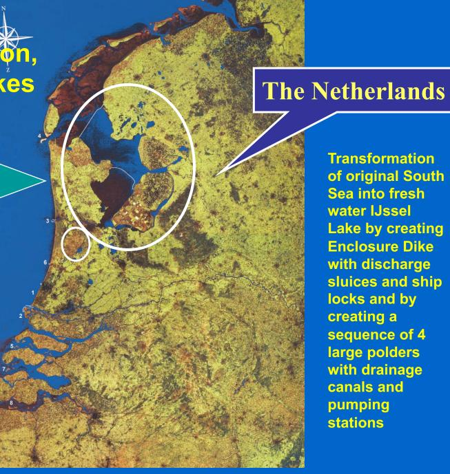
**Transformation** of original South Sea into fresh water IJssel Lake by creating **Enclosure Dike** with discharge sluices and ship locks and by creating a sequence of 4 large polders with drainage canals and pumping stations
